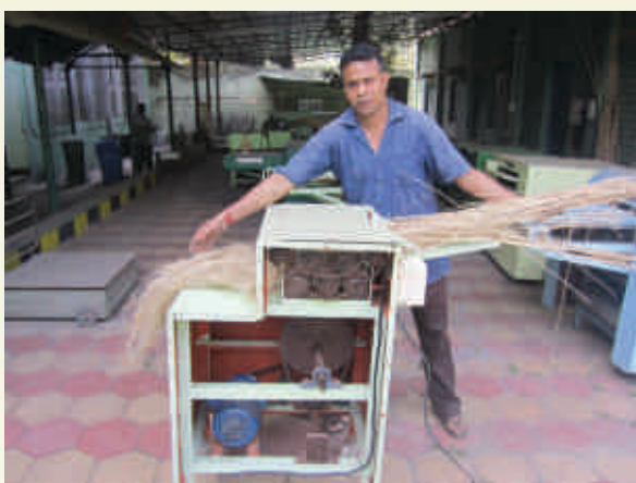
Figure 26: Developed flax fibre extractor and the extracted fibre, dried stalk and broken stalk
