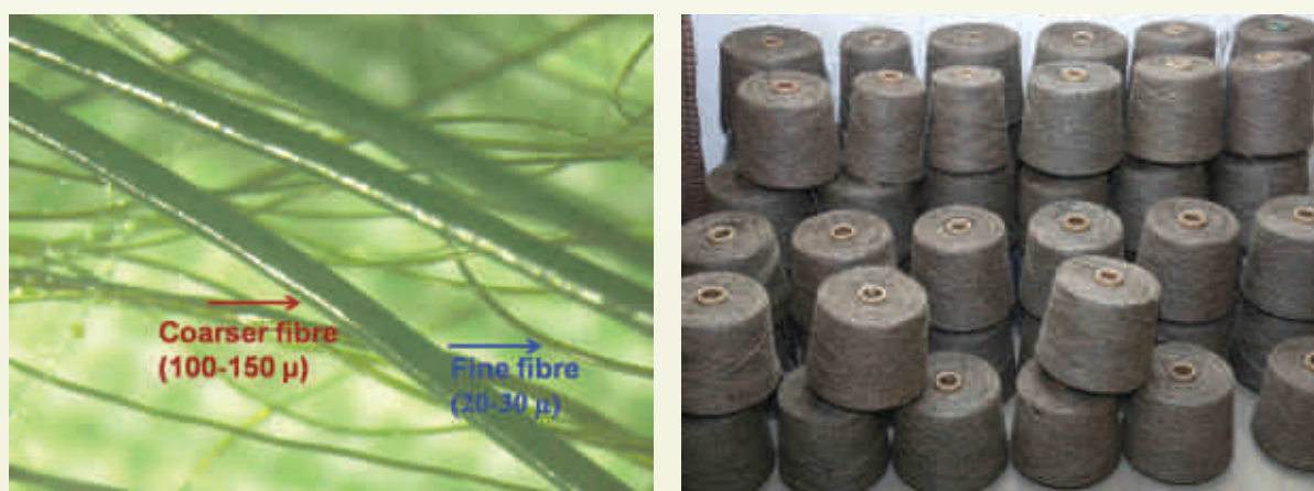
Figure 27: Microscopic view of coarser and fine yak fibres & Jute/yak (50/50) fibres blended yarn
