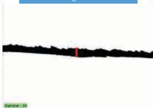
Figure MP-17.3: Measure the diameter of moving yarn in real time using video image processing and finally calculate CV (%)
