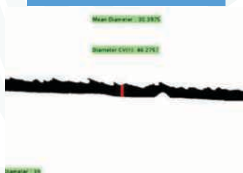
Figure MP-17.3: Measure the diameter of moving yarn in real time using video image processing and finally calculate CV (%)
