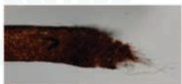
(b) Sunnhemp Thermal bonded fabric breakage: Adhesive failure
